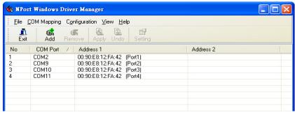
5. For Reverse Real COM mode, users should assign the TCP port number for the Remote Host/Server. Click the Configuration tab to modify the port number.
