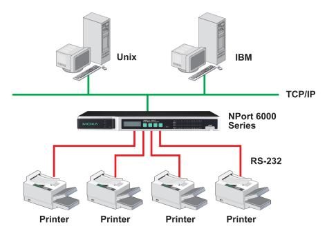
The NPort 6000's Printer mode provides an excellent solution for banking and stock exchange services with huge printing demands. Printer modes involve a network printer that is connected to a serial port on the NPort 6000, with a port number assigned to specify the printer's location. Windows or UNIX hosts can access the printer over the network in either RAW or LPD modes.
