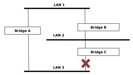
STP will determine which path between each bridged segment is the most efficient and then assign a specific reference point on the network. When the most efficient path has been identified, the other paths are blocked. In the above three figures, STP first determined that the path through Bridge C was the most efficient, and as a result, blocked the path through Bridge B. After the failure of Bridge C, STP reevaluated the situation and opened the path through Bridge B.
