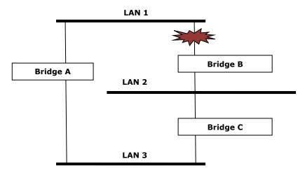
What happens if a link failure is detected? As shown in next figure, the STP process reconfigures the network so that traffic from LAN segment 2 flows through Bridge B.
