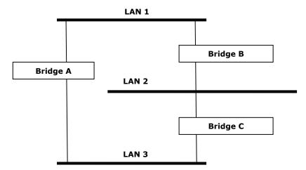
If STP is enabled, it will detect duplicate paths and prevent, or block, one of them from forwarding traffic. In the following example, STP determined that traffic from LAN segment 2 to LAN segment 1 should flow through Bridges C and A because this path has a greater bandwidth and is therefore more efficient.
