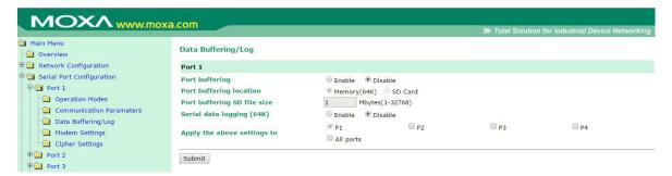
The NPort 6000 supports port buffering to prevent the loss of serial data when the Ethernet connection is down. Port buffering can be used in TCP Server mode, TCP Client mode, and Pair Connection mode. For other modes, the port-buffering settings will have no effect.
