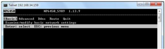
6. Use the arrow keys to move the cursor to IP address. Use the DELETE, BACKSPACE, or SPACE keys to erase the current IP address; then, type in the new IP address and press ENTER. Note that if you are using a dynamic IP configuration (BOOTP, SHCP, etc.), you will need to go to the IPv4 Configuration Field (or IPv6 Configuration Field) and press ENTER to select the appropriate configuration.
