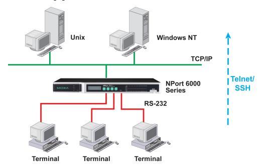
Terminal applications involve connecting terminals to UNIX or Windows servers over a network. A terminal connects to the appropriately configured serial port the NPort 6000, and the NPort 6000 transmits information to and from a UNIX or Windows server over the network through its Ethernet port. You may need to check with your network administrator to determine the appropriate terminal mode. All terminal modes support fast keys as used in many terminal applications.
