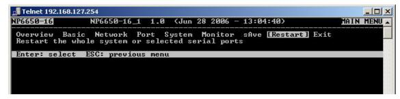
11. Press **S** or use the arrow keys to select **System**; then press **ENTER** to restart the NPort 6000.
