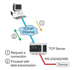
In TCP Server mode, the serial port on the NPort 6000 is assigned a port number which must not conflict with any other serial port on the NPort 6000. The host computer initiates contact with the NPort 6000, establishes the connection, and receives data from the serial device. This operation mode also supports up to eight simultaneous connections, enabling multiple hosts to collect data from the same serial device at the same time.
