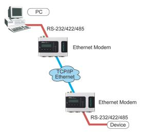
Ethernet Modem mode is designed for use with legacy operating systems, such as MS-DOS, that do not support TCP/IP Ethernet. By connecting the properly configured NPort 6000 serial port to the MS-DOS computer's serial port, it is possible to use legacy software to transmit data over the Ethernet if the software is originally designed to transmit data over a modem.
