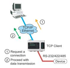
In TCP Client mode, the NPort 6000 can actively establish a TCP connection to a pre-defined host computer when serial data arrives. After the data has been transferred, the NPort 6000 can automatically disconnect from the host computer by using the Inactivity time settings.
