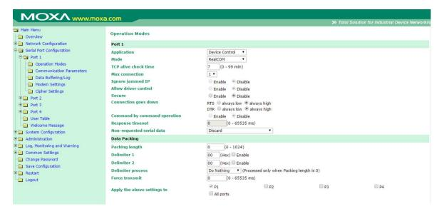
Select **Operation Modes** in the navigation panel to select and configure the mode for each serial port. For NPort 6000 models with two or more serial ports, you may use the checkboxes at the bottom of the window to apply the settings to one or more ports.
