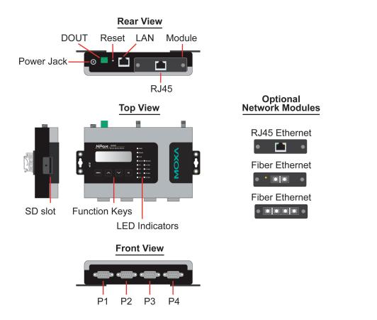
Note: The LCD panel is only available with standard temperature models.
