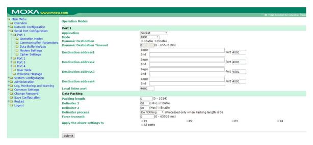
**Dynamic Destination (default=disable):** When enabled, the destination address and port number are decided by the source (IP address and UDP port number) of the last data received. When the function is enabled, you are NOT able to specify ranges of IP addresses for the serial port to connect to.
