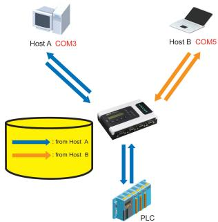
Once the PLC responds, the NPort 6000 will store the response in its buffer, decide that the response has been received, and then send back the command. The NPort 6000 will then be free to process the next command.
