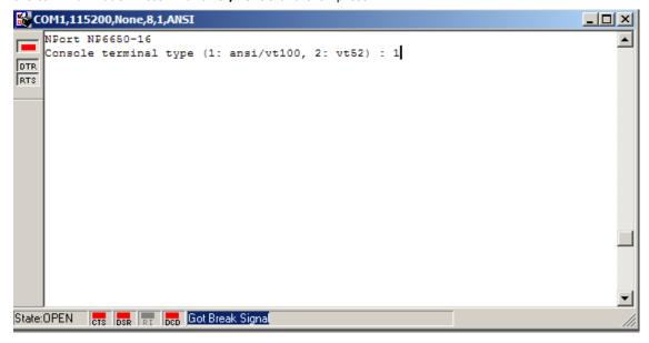
8. The main menu should come up. Once you are in the console, you may configure the IP address through the **Network** menu item, just as with the Telnet console. Please refer to steps 4 to 11 in the *Telnet Console* section to complete the initial IP configuration.
