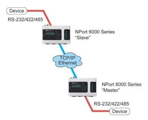
In Pair Connection mode, two NPort 6000 servers work together to remove the 15-meter distance limitation imposed by the RS-232 interface. One server is arbitrarily designated the master and the other as the slave—it does not matter which is which as long as there is one of each. One server is connected from its RS-232 port to the COM port of a PC or another type of computer, such as a handheld PDA that has a serial port; the other server is connected to the serial device through its RS-232 port.
