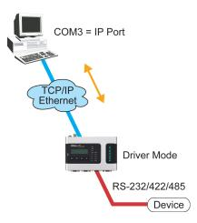
The NPort 6000 comes bundled with Real COM drivers for Windows systems and TTY drivers for Linux systems. Real COM mode includes optional data encryption, using SSL.
