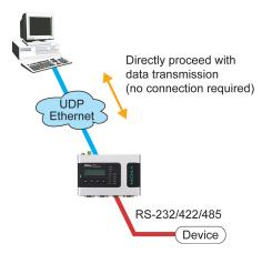
Compared to TCP communication, UDP is faster and more efficient. In UDP mode, you can unicast or multi-unicast data from a serial device to one or multiple host computers; and the serial device can receive data from one or multiple host computers. These traits make UDP mode especially suited for message display applications.
