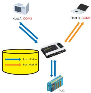
Once the PLC responds, the NPort 6000 will save that response to its buffer, assuming that the response is correct and then send the command back to the originator of the command. The NPort 6000 can respond in place of the PLC the next time it receives a request for the same command.
