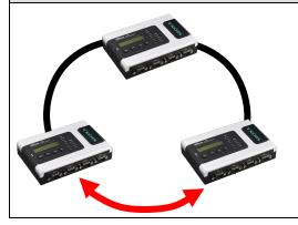
If there are 2N+1 NPort 6000 units (an odd number) in the Turbo Ring, with NPort 6000 units and segments labeled counterclockwise, then segment N+1 will serve as the backup path.
