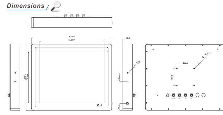
Mechanical 304 Stainless steel chassis(default), 316 Stainless steel Construction chassis(optional) Mounting VESA mount 100 x 100, Yoke mount for optional IP Rating Total IP66/IP69K 470 x 388 x 60 mm Dimensions Net Weight 9.5 kg
